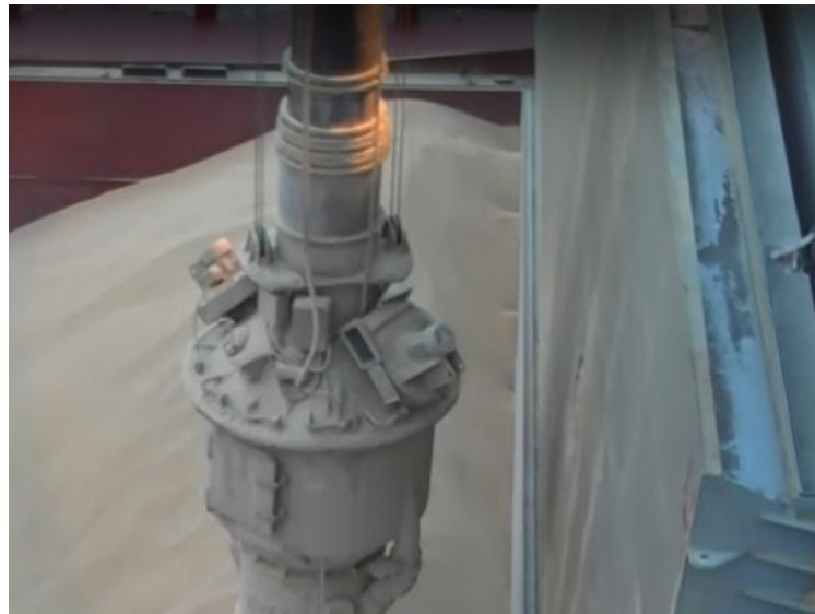
Figure 7. Grain flowing through the bleeder holes
